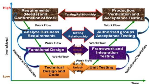
Fig. 6. V- Model of software testing.
