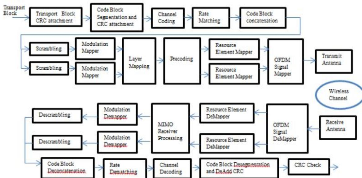
Fig. 2. PDSCH Transmitters and Receiver Structure [12]
