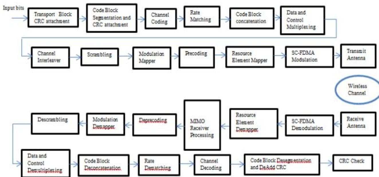
Fig. 3. PUSCH Transmitter and Receiver Structure[12]
