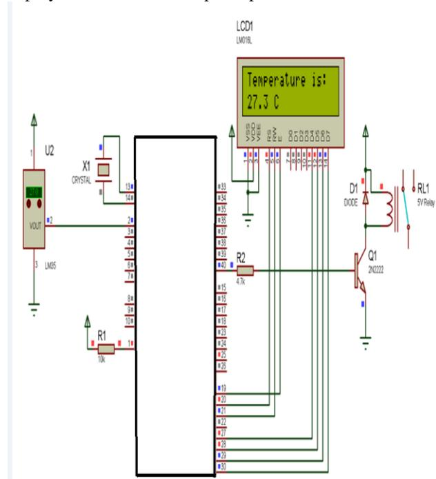
Fig. 1. Circuit Diagram For The Proposed Device
