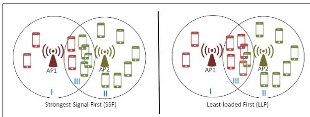
Fig. 2. Illustration of Existing Association Control Mechanisms
