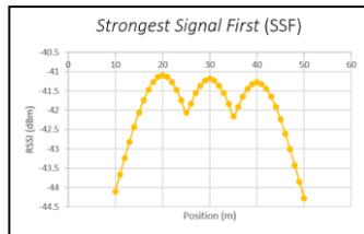
Fig. 8. RSSI received in all stations in SSF mode
